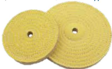
The blending capabilities of a sisal wheel combined with the polishing power of a treated muslin buff. Use this wheel to cut while removing scratches at the same time, works great with Black Magic compound. 3/8" wide spiral sewn.
