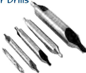
Center drills are used in a drill press, milling machine or lathe to start the hole to be drilled. The large body diameter and small drill size make them extremely rigid, thus eliminating any flex or 'walk' you will experience with other drills. Use to start the hole and to drill 'centers' on stock to be turned in a lathe.
