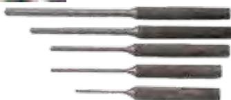
The special piloted point is designed to fit into the roll pins thus preventing damage to pin and hole during removal. The pilot can be 'ground-off' if desired, giving an extra long punch for removing long pins. Five piece set includes 1 each size.
