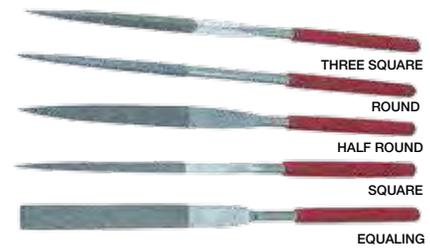
Fast cutting diamond files for ultra hard materials. 7 1/8" overall. Equalling file is 3/8" wide, 3/32" thick. Square is 3/16" wide. Half round cuts flat on bottom and is 3/8" wide. Round is 3/16" diameter. Three Square is 1/4". All sizes are approximate.
