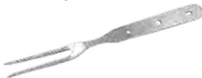
A perfect match for the SS822 carving knife. Bent and tempered, ready to handle and use. An extra long handle can be designed to make this an excellent Bar-B-Que fork. Great gifts. Fork is 11 3/4" overall, 7/8" wide .092 thick. Rivets or 1/8" pins and handle material are all that's necessary to complete this project.
