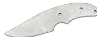
This hollow ground trail point blade is made from 440-C stainless. Overall length is 6 11/16". Blade length 3 1/2" x 1 1/2" at widest area. Approximately 7/64" thick, 3/16" pin holes are perfect for 5/16" cutlery rivets or 1/4" corby rivets. Kit includes blade, pins and handle material. Available sheath KT121.
