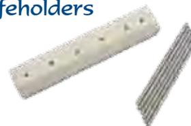
A must to make sure the blade is treated evenly throughout. These have high temperature removable pins that fit into holes pressed into a ceramic base, the pins hold the foil wrapped blades on edge so heat can circulate freely around each blade.
