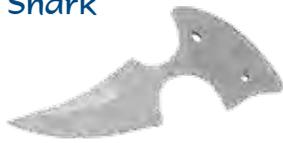
The Shark stainless steel specialty blade is easy to hold, easy to handle, easy to complete. Overall length 5 1/2", blade length 2 7/8", 2 3/4" wide at tang, 1 1/2" widest part of blade. 3/32" thick. Two pin holes for 1/8" pins or 3/16" cutlery rivets. Kit includes blade, handle pins and handle material.
