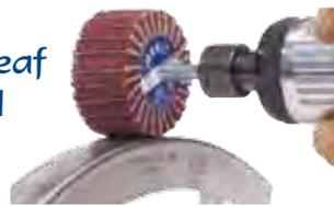
Standard X-weight abrasive cloth flap wheels are interleaved with Abrasotex for a softer and more flexible wheel. Used for deburring, producing decorative finishes, removing fine scratch lines and rust removal. Produces a finer finish than regular flap wheels. 3" x 1" with 1/4" arbor. Maximum rpm 12,000.
