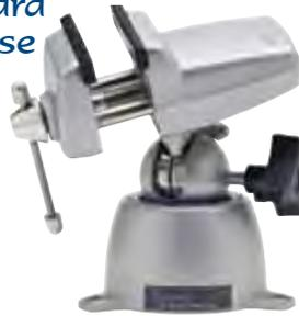
The Standard PanaVise gives you a complete range of adjustments to suit your needs. With rotation through 360° and 180° tilt, PanaVise provides the perfect angle on any job. This vise opens to 2 1/4" with 15/16" throat. 2 1/2" nylon jaws can withstand continuous heat to 200°F. Head removes easily from base for additional use when grinding, polishing or drilling those hard to grip pieces.
