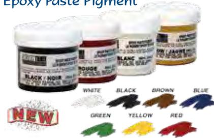
Pure, dry, colored pigments can be used alone or mixed to produce additional colors to suit any project where color is desired. Add the paste to the epoxy resin then measure that mixture in the proper ration with the hardener. Use a maximum of approximately 10% volume pigment paste to combined resin and hardener. To maintain the same color over several projects, mix a master batch of color with resin and store for later use - only add hardener when you are ready to use.
