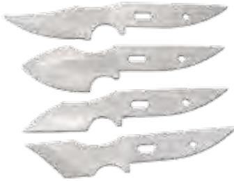
Four piece set of the most used wood carving blades. We added this set for the woodworkers who want to make their own handle for a custom feel. Sold in sets only. 440-C Stainless. Overall length of each 4 1/2" - 5". Slot wood to proper angle to insert blade and fasten with 1/8" pins.
