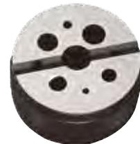
Block is made from a steel forging and is hardened and ground. Smooth finish on the face preserves finish of work being held. Base is recessed to make it light and yet strong. Approximately 1 1/2" high and 3" diameter. Holes vary in sizes from 1/8" to 5/8". *Made in the USA.*
