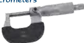
Precision micrometer with .001 graduation. Carbide face anvil and spindle is hardened and ground with micro-lap finish on ends. Complete with wooden box.
