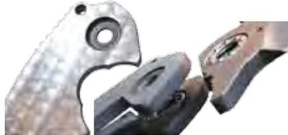
The illustration (above left) shows the pocket in the left liner once the procedure has been completed. The first bearing will fit in this pocket. The second pocket should be cut in the blade. In final assembly (see above right), the liner pocket and blade pocket should be facing up when the knife is in the proper position for assembly.
