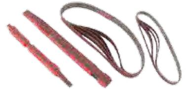
Perfect for hand finishing knife blades, actions and other flat surfaces, it stays flat and 'ripple' free. Detailed, hard to reach areas are a snap. The easy to use tapered plastic stick holds a replaceable sanding belt. The patented spring loaded mechanism allows belt to rotate 360° guaranteeing use of entire belt. Two sizes, 1/4" x 6" long or 1/2" x 8" long. Each comes with 5 belts (1 each grit). Replacement belts are sold in packages of 5 all one grit.
