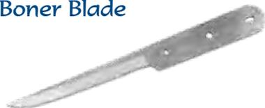
Wide handle and sharp, narrow blade, easy to hold, easy to use. Shape handle to fit the hand of the user. 10 1/8" overall, 5 1/2" x 11/16" x .100 thick. Use cutlery rivets or 1/8" pins.
