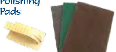
A super strength nylon pad impregnated with abrasive. Resists tearing or shredding, won't rust, folds easily to any size, conforms to any shape or surface. Use to remove fine burs, rust and corrosion, clean, polish stainless to a satin finish. Rinse and save to use over and over wet or dry. 6" x 4 1/2" holder uses 1/2 of standard pad.
