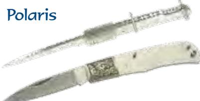
Embossed Nickel Silver bolsters attached to Stainless Steel liners, elegant filework on the top edge of the mirror polished AUS-8A Stainless and locking lever are special features of this lockback folder. 6-1/2" overall open, 3-3/4" x 1" when closed. 2-1/2" cutting edge. Minimum handle material size: 7/8" x 2-3/4" x .135". Requires TD40, TD49 and TD21 drills.
