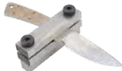
This versatile tool can be used for holding your knife blades to do complex file work, filing slots for guards to reach angles needed when hand sanding your blades. Our file guide is precision machined and ground from A-2 tool steel and hardened to 62RHC for long wear. Overall length 3.250", maximum blade width 2", each jaw is 3/8" x 3/4". Made in the USA.
