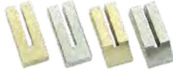
Guards made especially for the Hi-Polished blades #SS458, SS461, SS495, SS783 and SS782. Milled from 3/8" x 3/4" x 1 3/4" bar stock, slotted .160 x 1 5/16" long. Available in Brass or Nickel Silver, with or without finger groove.
