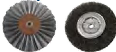
DX16463 Brush away rust, scale and dirt with ease. WW612 Wire wheel is 6" in diameter. 1 3/4" long, .008 diameter crimped wire, 9/16" face. The carding wheel has .003 diameter wire for fine work The 1/4" arbor hole can not be drilled larger.
