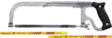
Hacksaw frame is corrosion proof, polished nickel with 3 3/8" throat, adjustable for 10" or 12" blades. Molded plastic handle. Blade holding bolts are adjustable to four positions. Rear bolt has wing nut for easy tensioning of blade. Comes with one carbon steel blade.
