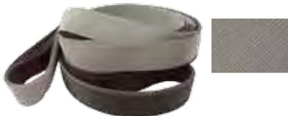
Extremely flexible and sharp cutting. Rayon cloth backing and an added aid for cooler grinding. The special 'pyramid' structure allows layer upon layer of the grit to expose itself as you grind, resulting in a consistent grind from start to finish.
