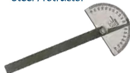
Preferred by machinists for setting bevels, measuring, and transferring angles. Made of ground stainless steel. Graduations from 0 to 180° in opposite directions. 3 3/8" x 2" head. 6" adjustable protractor arm locks into desired position with knurled thumb nut.
