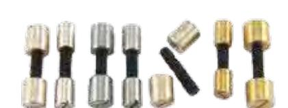
"Three piece rivets." Each nut is drilled and tapped 3/16" deep, adjust length by shortening the bolt as necessary. These rivets give an extra neat finished appearance. Also known as Luke Rivets.
