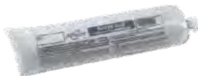
The finest greaseless compounds available anywhere. Builds up a good head and remains on the wheel. The aluminum oxide grit is of uniform size, therefore cutting clean and sharp. These compounds work well on all muslin and felt wheels. Keep tightly sealed, refrigerate if possible. Shelf life six - eight months. Approximately 2 lbs. each.
