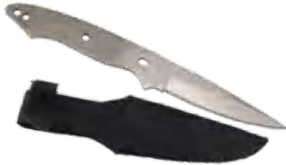
False top edge and thumb notches on this stainless steel blade. Kit contains three 3/16" brass pins, handle material, blade and Nylon sheath. Overall length 8-3/4", blade is 3-1/2" x 7/8" wide x .108" thick.
