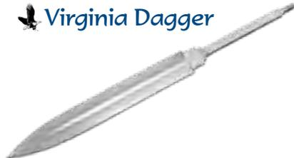
Hollow ground mirror finish blade. 6A High Carbon Stainless Steel. 13 1/2" overall, 1 1/8" wide, 8 3/4" double edge blade, approximately 3/16" thick. Tang is threaded 6x1mm.
