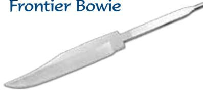
The Frontier Bowie Blade is made from 440C Stainless cutlery steel, satin brush finished, sharpened to a fine edge and designed for a hidden-tang handle to be added. 10-1/8" overall, the blade is 5-1/2" x 1" x 3/16" thick. Kit includes blade, unshaped guard, pommel and pre-drilled handle material. Available sheath KT914.
