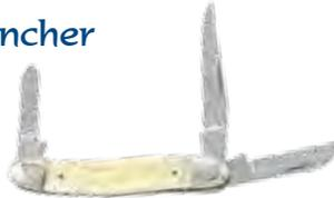
The Rancher stainless steel 3-blade folder measures 3 1/4" long x 1/2" wide when closed, it easily fits in your pocket. 2 mirror polished blades measure 1 1/4" another is 2 1/4", hardened, tempered to hold a fine edge. The nickel silver bolsters are attached to the brass liners. Kit includes all components except handle material. Requires drills #TD47 and #TD0625.
