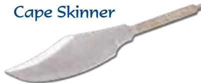
This deep-bellied skinner blade is skillfully crafted and ground from the finest 5/32" 440-C stainless cutlery steel. Overall length is 10-1/4", blade is 5-1/2" x 2" wide. Kit includes blade, guard, pommel and pre-drilled handle material.
