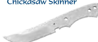
Skinner 8 1/2" overall, 9/64" thick, predrilled for #CP600 corby type rivets and #CP500 thong hole tubing. Blade length 3 1/2" x 1 1/8" wide. Available sheath KT115.
