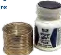
Use Safety Silv 56 to make repairs to mild and stainless steel, nickel, brass and copper parts when high temp soldering is necessary. The fluidity of Safety Silver 56 promotes penetration into the joint. The Silver colored braze matches well with stainless steel. Flows around 1200°, cadmium free. 2 oz. white flux and 1 oz. solder.
