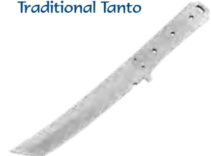
Traditional Tanto style blade, the upswept tip and wide handle make this blade stand a cut above. Pre-drilled with three 3/16" tang holes and two 3/32" bolster holes. 12 1/2" overall, the blade is 6 1/2" x 1 3/16" wide and 3/16" thick.
