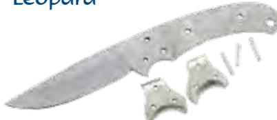
The Leopard is a mirror polished blade with tapered tang. Comes with the pre-shaped nickel silver bolster and 3 pins for attaching bolster to blade. Ground from 8A stainless steel this blade measures 8-1/2" overall, blade is 3-1/2" x 1" x 5/32" thick. Has two 1/8" holes for pins or mosaic pins and one 7/32" hole for thong tubing or mosaic pin. Available sheath KT102.
