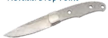
Hollow ground from high carbon stainless, satin finished, drop point blade with 1/8" thick nickel silver bolsters attached and a tapered tang. Easy to complete with handle material of your choice, Mosaic pins will add an extra special touch to this all time classic. 8" overall length, 3-3/8" blade, 1" wide, 5/32" thick. Two 1/4" tang holes for handle, one 1/4" thong tube. Kit includes blade, 3/16" nickel silver pins and handle material. Available sheath KT104.
