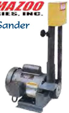
1/3 HP motor, 1PH, 1725 RPM. 4" contact wheel, tilt table. Vertical sander. 1800 SFPM. Platen can not be removed. **Actual shipping charges apply.** Use 1" x 42" belts.
