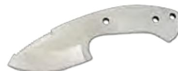
The 1 3/4" crush-ground serration on the top edge of this 3/16" thick blade makes for a most unusual skinning knife. 7 1/2" overall with 3" x 1 3/4" wide blade. Predrilled for 2 #CP600 corby type rivets and CP500 tubing. Although a guard is not required, you can use 3/8" x 3/4" bar stock and solder a bolster on for a different effect if desired. 440-C Stainless. Available sheath KT113.
