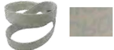
A super fast cutting abrasive belt for precise, uniform, close-tolerance finishing. The high-strength 5 mil polyester film backing is extremely flexible for contour work. This super thin belt is resin-bonded for durability. Use on all your knife parts, steel, brass, nickel, wood, plastics even leather.
