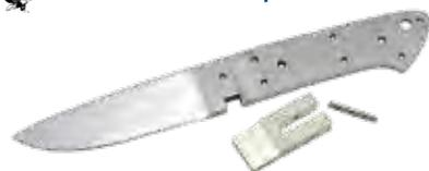
The Delaware Drop Point is ground from 440C stainless steel. With excellent wedge grinding, a deep mirror finish, and tapered tang, the custom drop point has earned its name. With a 4" blade and a 3 1/2" cutting edge, this blade is 7/32" thick, and the tang tapers to 3/32". The tang has six 3mm and two 4mm holes. Available sheath KT111.
