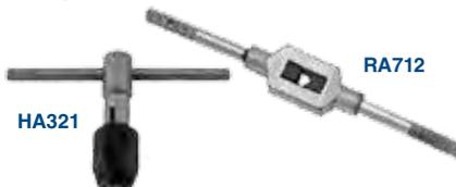
Sliding handle with spring tension stop. May be extended to full length in either direction for more leverage. Has positive grip knurled nut. HA321: For #0-1/4" taps, with extra stepped recess in chuck providing smaller jaw capacity to hold #0-#10 tap. RA712: For #0-1/4" taps and for our 700 series pin reamers. Overall length 5".
