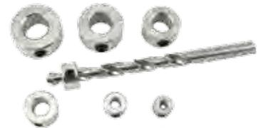
Takes the guess work out of drilling! Just slip the collar over drill bit; measure desired depth; then tighten set screw. Will drill to uniform depth every time. Steel collars will not slip like plastic stops. Slotted screws tighten into flute. "Rust-Proof" plated finish. 7pc. set with one collar to fit these drill sizes: 1/8", 3/16", 1/4", 5/16", 3/8", 7/16", 1/2".
