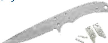
The tapered tang and false top edge make this graceful design one of our best. Mirror polished 8A stainless steel blade comes complete with a nickel silver bolster and 2 pins. Overall length is 7-3/4", blade is 3-1/2" x 7/8" wide x 9/64" thick. Drilled with four 2mm handle pin holes and one 7/32" thong hole. Available sheath KT104, KT231.
