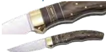
After the handle is final sanded, seal with a thin coat of the 3M instant adhesive or Zap-a-Gap to seal, then final polish. This will add a protective coat and seal your mosaic material.
