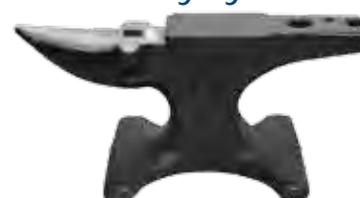
Quality alloyed castings, our 70 lb. anvil is precision milled and heat treated. 4" x 6" face, 3 1/4" x 8" horn and 3 1/4" x 5" heel. Height 8 3/4", base 11" x 9". Perfect for forging Damascus.
