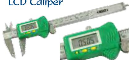
Stainless steel hardened frame with graduated scale and thumb roll. 4-way measurement: inside, outside, depth, step. Accuracy .001 per 6". Has a large LCD display window for easy reading. Inch/metric conversion or reading at the switch of a button.
