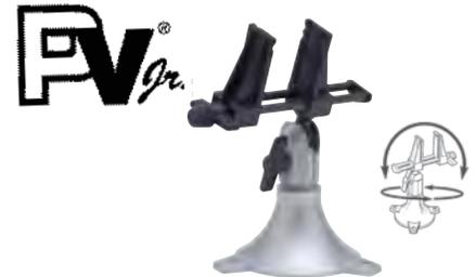
PanaVise Jr. uses the famous PanaVise design that tilts, turns, twists and rotates. One quick turn of the control knob and you securely position your work exactly where you want it. Overall height is 6 3/4", weighs 1 lb. 4 oz., head rotates and swivels 360 degrees, pivots 210 degrees. Jaws are 1" wide and 2" high, opens 2 7/8" and are made of fiber reinforced thermal plastic alloy. Will stand continuous heat up to 350 degrees F (intermittently up to 400 degrees F.)
