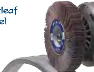
Rated at 6000 max rpm optimum performance is obtained by running these wheels slower than the maximum rpm. 6" x 1" x 1". X-weight abrasive cloth flap wheels are interleaved with Abrasotex for a softer and more flexible wheel. Used on your buffer or grinder for deburring, producing decorative finishes, removing fine scratch lines and rust removal. Use arbor bushings listed below.
