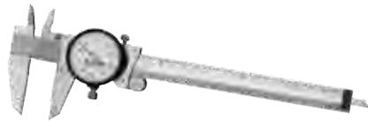
The only dial caliper made in the USA. Full six inch range, four-way stainless steel dial caliper with knife edge contacts for inside and outside measurements. Readings taken directly from the bar and dial indicator. Measurements with one hand, thumb roll for fine adjustment. Knurled thumb screws lock the moveable jaw and adjustable indicator dial at any setting. English model dial indicator graduated .001" with .100 range per revolution. Case included.
