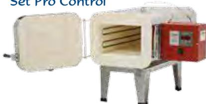
Set-Pro with Express Mode, easy to use 3 button temperature control. Control up to 8 separate temperature points per firing. Store up to 4 individual programs each capable of holding up to 8 segments. "On-the-Fly" features allow you to add time and temperature to your holds along with a skip ahead feature.
