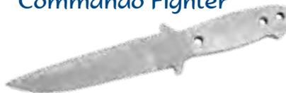
Heavy 3/16" thick fighting blade is 9 1/2" overall, with 4 3/4" x 1 1/8" wide blade section. Upper 3 1/2" false edge and cross guard. Extra heavy tang is drilled for two CP600 rivets and CP500 thong tubing. Use the CP607 brass to form a contrasting guard if desired or shape the handle material to conform to the pre-formed cross guard. Available sheath KT111.
