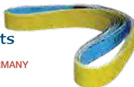
Our J-Flex belts are flexible, aluminum oxide material. Great on contoured workpieces. Use on your stainless and high alloy steels as well as on all ferrous and non-ferrous metals. The semi-open coated material is resin bonded with a special gold colored top coating to aid in cooling and to resist loading.
