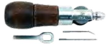
Automatic sewing awl, for leather, canvas and other similar materials. Sews an automatic lock stitch just like a machine. Comes with a 12-1/2 yard spool of black polyester waxed thread on the handle, one straight and one curved diamond point needle, wrench, instructions. Extra needle and wrench store neatly in hollow handle.
