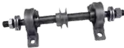
Ball Bearing double-end mandrel features two high-quality precision grade die-cast ball bearing pillow blocks. Will run wheels up to 1" thick. Use with flap wheels, wire brushes, buffing and grinding wheels having a 1/2" arbor hole. Our keyless chuck can be mounted on the right hand end to allow use of various accessories such as sanding drums, mounted points, etc. Pulley diameter 2", shaft diameter is 5/8" threaded 1/2"- 20 Right and left hand, 12" overall. **MADE IN THE USA.**
