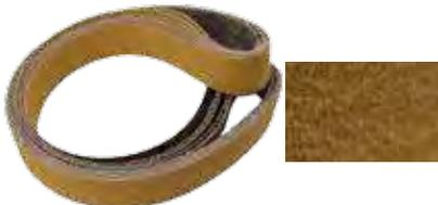
Premium Cubitron™ abrasive grain YF weight water resistant polyester cloth backing for heat resistance. Features grinding aid for cooler grinding. Extremely long lasting and fast grinding. Great for grinding heat sensitive alloys such as titanium, stainless, nickel and cobalt. For dry applications only.
