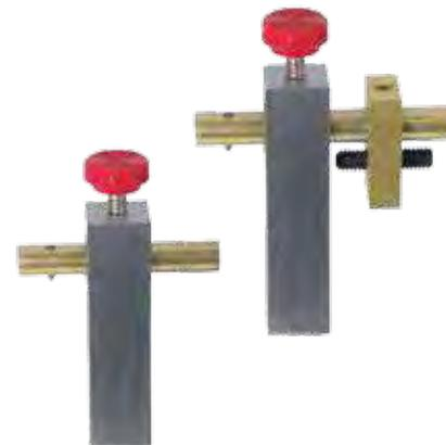
Use this handy tool to scribe the center lines as a guide for grinding knife blades. Designed for accuracy, this scribe can be adjusted from 0-1/2". Adjusts 1/32" per revolution using fine adjustment screw. Replaceable carbide tip marks even the hardest knife steel.
