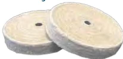
Made from full-disc 3/8" spiral sewed muslin sections glued together with a canvas disc cemented on each side to prevent edge breakdown. A hard wheel that produces aggressive cutting action when greaseless compound is applied. Wide face gives greater surface contact and a smooth metal removal.
